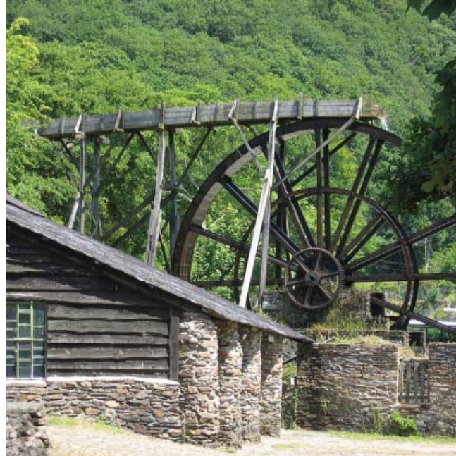
Clockwise from left: Electric mine tram with visitors approaching the George & Charlotte Mine (K. Prisk © Cornwall County Council); Overshot waterwheel formerly used to power a manganese ore-crusher at this location (A. Cocks © Cornwall County Council); Morwellham from the air showing the Great Dock (left) built for additional copper ore storage in 1859 (B. Gamble © Cornwall County Council)
