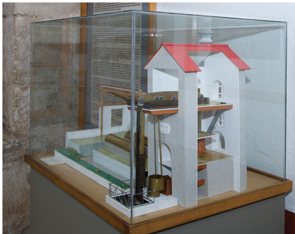
A model of a Cornish beam pumping engine within the visitor centre at Mina Acosta, Real del Monte
