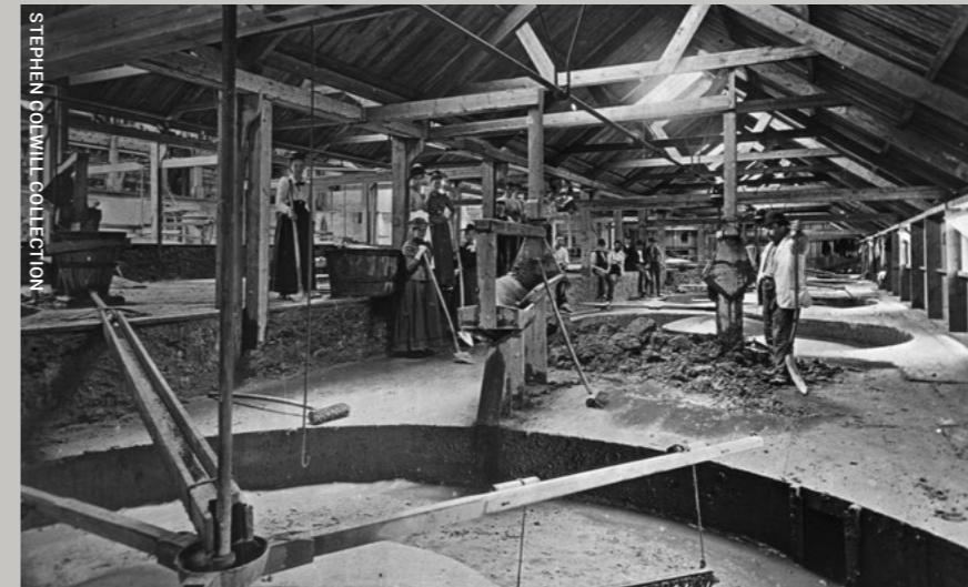
Workers on the buddle floors of Dolcoath Mine, Camborne, circa 1910. The female workers appear particularly well dressed in this excellent photograph
