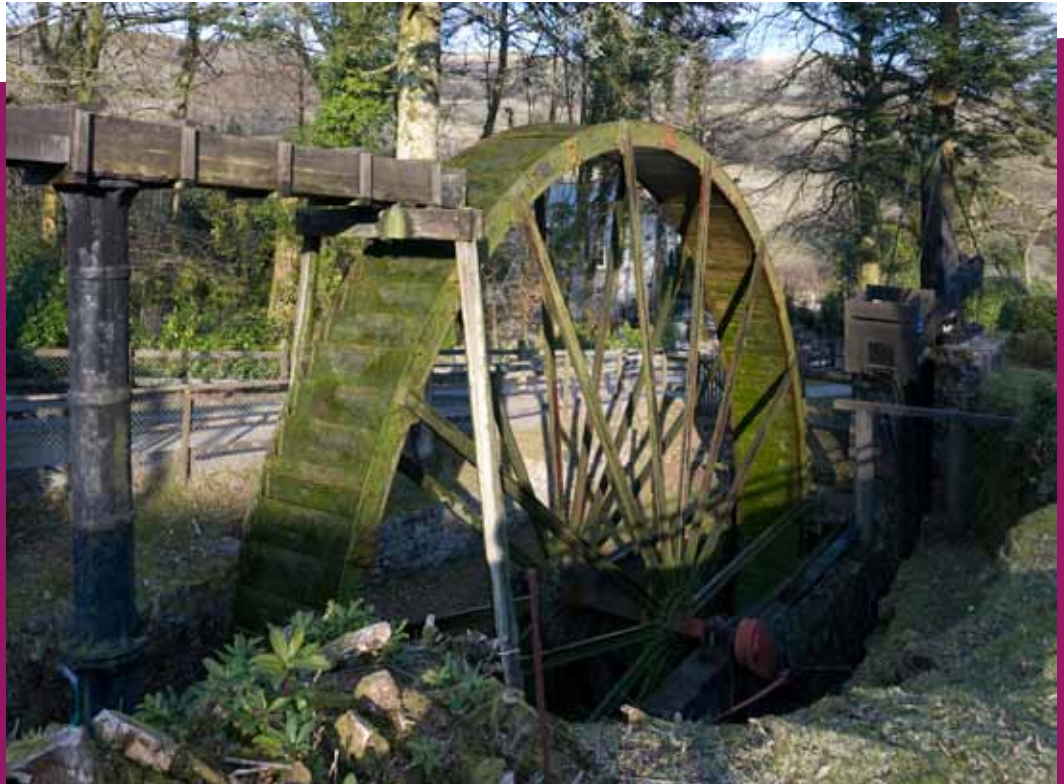
Right: The 35ft (10.6m) water wheel at Wheal Martyn China Clay Museum, near St Austell.
